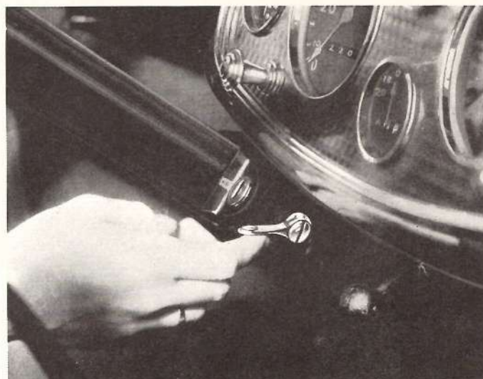
Automatic Starting which eliminates starting pedal and prevents the engine from stalling.
