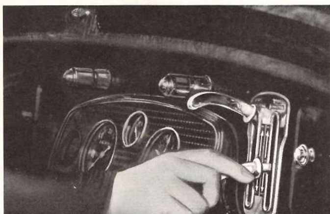
Improved Free Wheeling in all forward speeds is effected without touching the clutch. The change from Free Wheeling to conventional gear is made by depressing the clutch and putting the instrument board control down.
