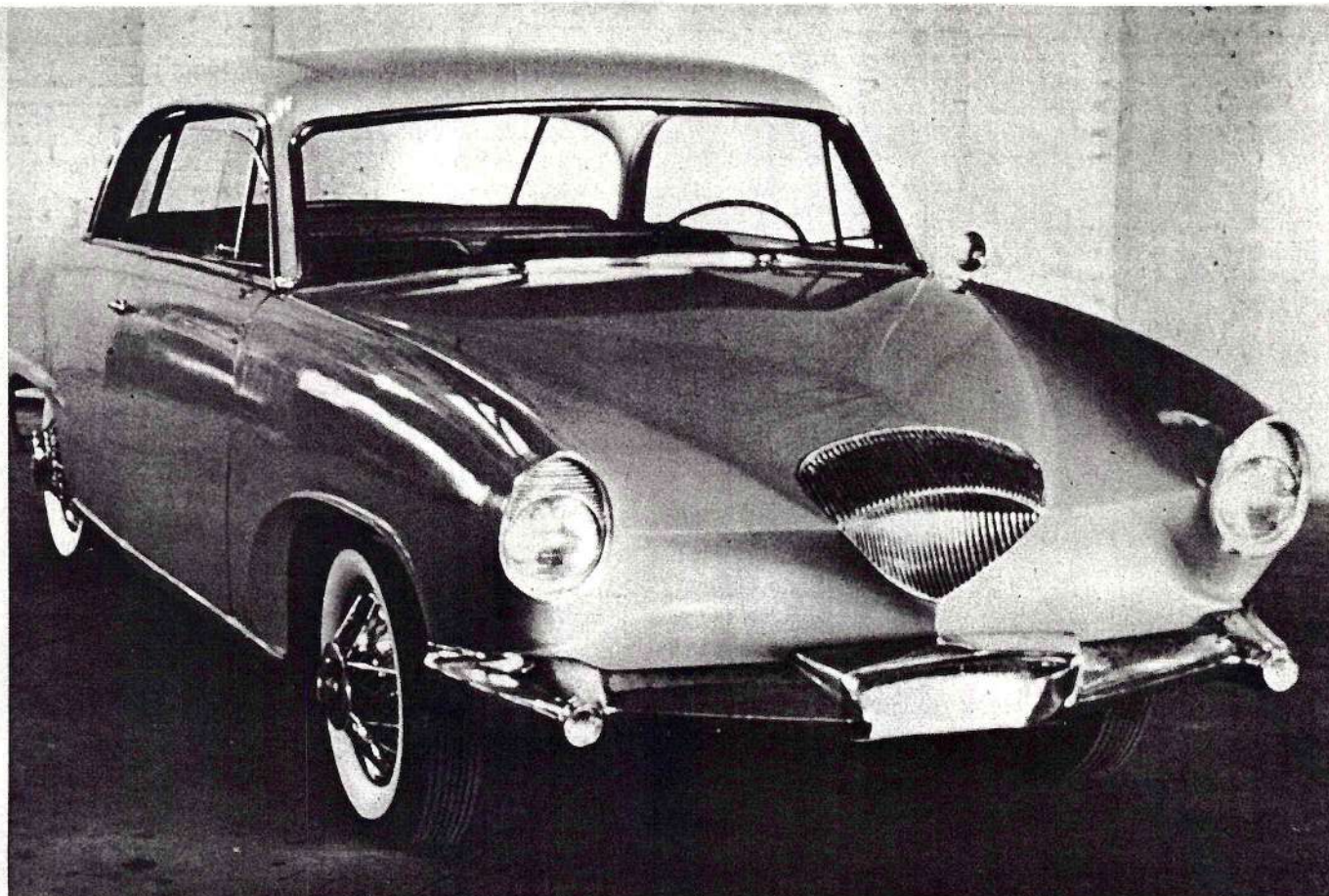
Howard A. (Dutch) Darrin restyled the 1955 Willys Aero Eagle by building up and stretching the fenders and hood but left basic body alone. Constellation ("kiss mouth") grille and front smack of Kaiser-Darrin roadster, which Darrin also styled. Prototype shown would have become 1957-58 Willys.
