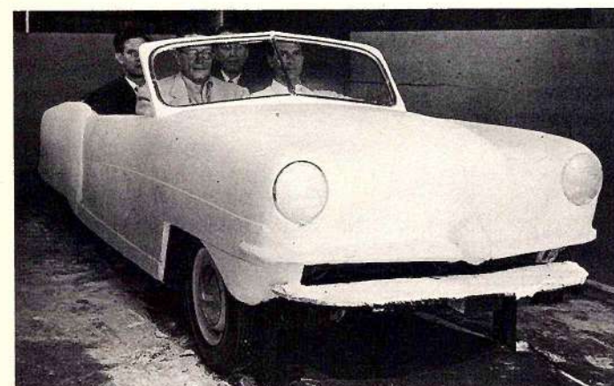
Fiberglass shell for one of Darrin's K-F econo-car proposals with Dunc McRae "driving," Dutch in the front seat, K-F's Zimmerly and Lindbergh in the back. Similar design was later proposed to Crosley.
