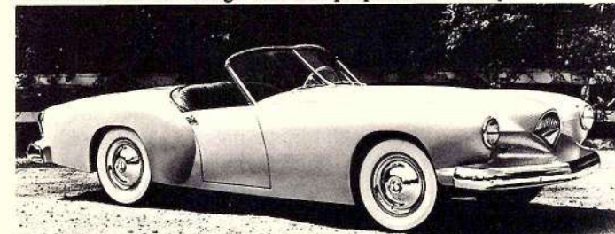
The Darrin as Dutch wanted to build it. The lower headlights and lack of "bananas" on the bumpers are the main changes from the production car.
