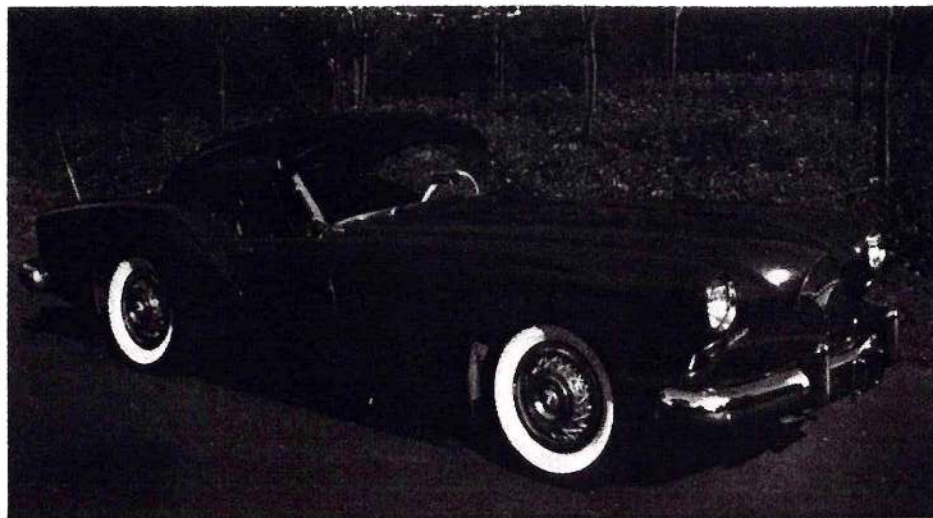
It is believed that Darrin designed this little bardtop coupe for his own personal use. Kaiser Darrins were noted for their sliding doors, the pursed-lip grille, and the curved one-piece windshield. Several of these cars were fitted with McCullough superchargers. (Darrin Collection)
