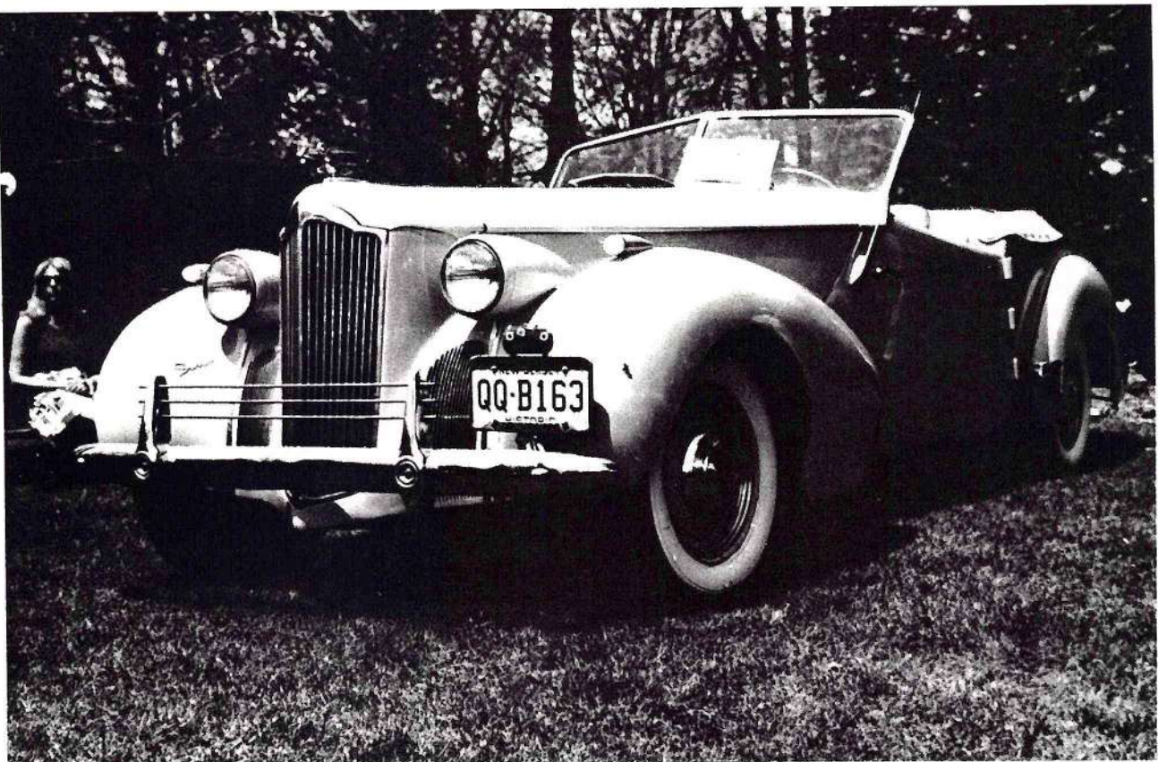
Please note the small differences in these two Darrins. Above, a 120, and below a 180. Bumpers, grille guards, and bumper guards differ. The grille bars on the 120 are stationary, whereas the 180 has thermostatically controlled shutters . . . Hood ornaments differ . . . The 120 has no hood louvers, the 180 has chromed louverstrips. The wire wheels on the 180 are monogrammed Darrin.
