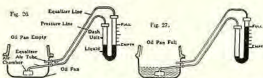
Fig. 26 (left). Oil level Telegage in operation. Oil pan empty. Fig. 27 (right). Oil level Telegage in operation. Oil pan full.
