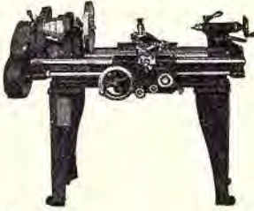
Fig. 9. This lathe can also be supplied with milling attachments, and keyway cutting attachments.
