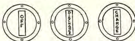
Fig. 19. Battery indicator showing its three indications.
