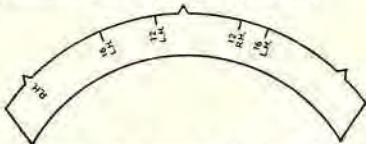
Fig. 29. The markings shown on this sketch are for the V-12 and the V-16 as well as for the V-8 engines.
