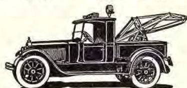
Fig. 58A. Shows how the wrecking crane is intended to be attached to the rear of a service car.
