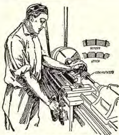
Fig. 17. Dressing down a commutator on a lathe when it is very rough or pitted, or when mica protrudes above the commutator bars. Use a sharp tool and fine feed and take light cuts. Remove all copper or solder which may bridge segments and polish with sandpaper (not emery cloth). Holes in commutator segments can be filled with a paste made of glycerin and litharge, which will harden in a few hours.
