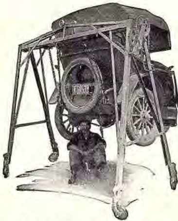
Fig. 41. A portable hoist. This hoist is composed of steel angles thoroughly braced. The top frame is in the form of a standard bridge truss.
