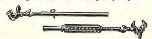
Fig. 56. Towing pole. With this device a car can be pushed or pulled. This towing pole supplies a rigid connection between towing car and disabled car, which prevents jamming on sudden stops or down grades.
