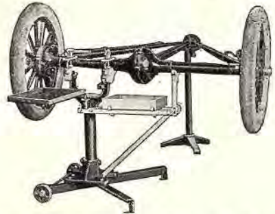
Fig. 44. Ford-Chevrolet axle stand. The engine stand (Fig. 42) is converted into an axle stand by removing two cap screws, releasing the clutch and fitting assembly, and applying to the yoke the two clamps. A collar is placed over the upright to support the grease pan and outboard support. Separate support is included for torque tubes. It is adapted to all types of split rear axles and to any front axle.
