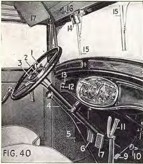
Fig. 40. Driving compartment of the Cadillac V-8 series "355" car showing instrument board, control levers and pedals. The Cadillac V-12 series "370," and V-16 series "452" driving compartment, instrument board and controls are similar except the accelerator pedal and the location of the spark control and the cigar lighter.
