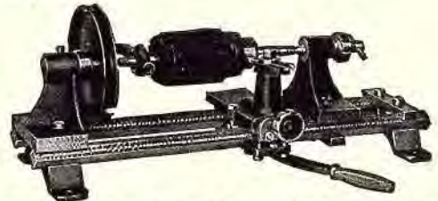
Fig. 10. The turning tool is controlled by a hand-wheel screw feed—the carriage is operated lengthwise by a drop-forged handle with suitable adjustment for every commutator. The lathe is built with 7" swing; bed 22" long; furnished with two Armstrong high-speed tool bits, lathe dog, suitable wrenches, etc., and is complete, ready for operating. It is driven from any available power. Shipping weight complete, 35 lbs.
