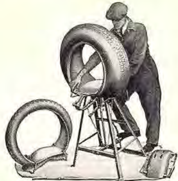
Fig. 44A. Tire spreader, designed to spread casings for inspection and to hold casing spread while being repaired. When foot lever is released casing assumes its original shape. When break is located, casing is inserted under the four hooks of the detachable buffing plate and casing thus permanently spread, can be removed for buffing and stripping.
