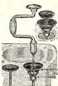
Fig. 64. The McCullough valve reseating tool consists of a carborundum cloth cone held to the face of the valve as shown. The valve is used just the same as a reamer, the cloth cutting the seat in the valve seat of cylinder at the same bevel as that of the valve-face. Emery cloth or sandpaper will do quite as well, but will not last as long.
