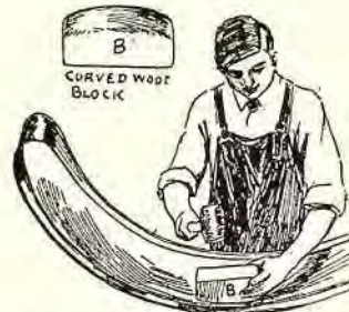
Fig. 45. Easy method of removing dents from fenders with the use of a shaped wood block.
