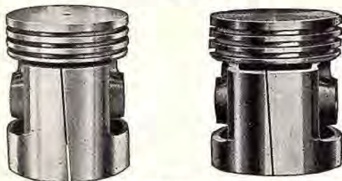
Fig. 1. Aluminum-alloy pistons of the constant clearance type with a split skirt. Pistons of this type can be given less clearance. With the use of aluminum pistons which cool readily, the use of larger valves and higher compression is permissible.
