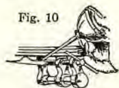
Fig. 10. Lubricating the surface of the separated spring blades. Fig. 11. The same tool used as a temporary clamp to secure a broken spring. Fig. 12. The spring tool.
