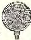
Fig. 27A. A special gauge designed for testing the comparative pressure of each cylinder, called a compressometer. 1 Tells whether compression is uniform in all cylinders—whether piston
