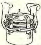
Fig. 31. One method of slipping a ring on a piston and into the groove. Take three strips of sheet metal, brass or tin (S), for instance, about 1/32'' thick, 1/2 wide, and 5" long; bend these at right angles and hang them on the edge of the piston at equal distances apart. The ring (R) may then be slipped over these skids till it is opposite its groove, when the strips may be removed and the ring allowed to slide into place. Install the ring in the lower groove first and work to the top groove last. The same strips may also be successfully used in removing the rings.
