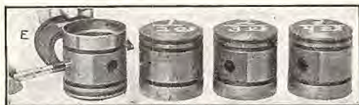
Fig. 26. Miking and chalk marking pistons.
