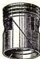
Fig. 2. Note the spiral slot which, the manufacturers claim, controls expansion and contraction due to changes in engine temperature thereby maintaining a constant clearance. The spiral slot also assures constant lubrication between piston and cylinder wall therefore decreasing wear.
