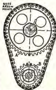
Fig. 64. The marks on the cam-shaft gear (A) should line up with those on the crank-shaft gear (B) before the gears are removed, and should be replaced in exactly the same position. Note the arrow points on chain.
