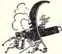
Fig. 20. Removing grease from under fabric brake lining on a two-piece internal expanding brake shoe.
