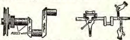
Fig. 25 (left). Scored crankshaft bearing pin. Note the ridges. This is only a slight score.
