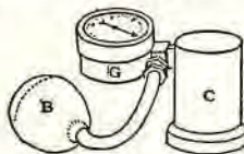
Fig. 76B. A valve-tester. To test, drop valve in seat without valve spring; place cup (C) over valve; pump air pressure with bulb (B). If valve leaks, hand on gauge (G) will fall back; if valve is tight hand will hold steady.
