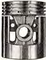
Fig. 2A. Nelson-Bohnalite piston of an improved light alloy design of the narrow-steel strut type (do not confuse with the "wide-steel strut type"). This piston differs from the split-skirt type, as it is made with special alloy steel struts so placed in the piston that they control expansion and maintain satisfactory clearance under various engine operating conditions. With well-finished cylinder bores, these light alloy pistons are fitted with less clearance than is used in fitting cast-iron pistons. 2
