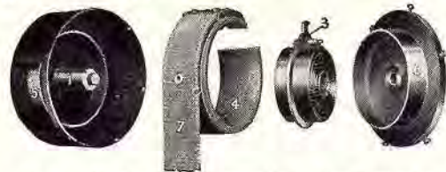
Fig. 53. Showing parts disassembled. First illustration at left is the cover assembly; next, shoe assembly; next, spring assembly; next, base assembly.
