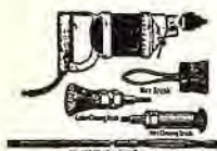
Fig. 76A. A typical carbon-removing set. The parts, from top down, are as follows: portable electric drill, wire brush for general carbon removal, wire brush for removing carbon and burnishing cylinder head, wire brush for removing from sides and bottom of port hole, wire brush for cleaning valve-stem guides. (The outfit shown is made by Temco Electric Motor Co.,
