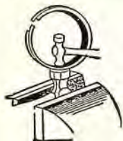
Fig. 18. Peening a piston ring. It is very important in any peening operation that the surface upon which the hammering is done be as flat and hard as possible, for any irregularities in the shape of the surface plate will be just as effective in causing distortions as a blow from a badly shaped hammer. One method of providing such a surface plate is shown.
