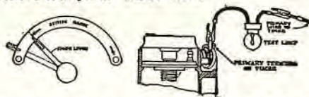
Fig. 65 (left). Position of the spark lever, when timing the ignition. The end of the lever on the quadrant should line up with the point of the arrow, as illustrated.
