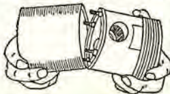
Fig. 3. The Marmon two-piece piston (1920-1926) is a combination piston: the head and body are aluminum, and the skirt is cast iron. A .0025" to .003" clearance was given. The one-piece piston was later used by Marmon.
