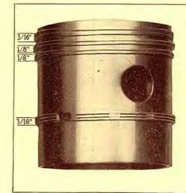
The new pistons are fitted with three compression rings above the pin and one oil regulating ring below
