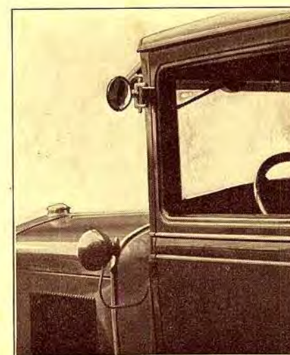
This mirror, with its universal mounting on the door hinge, gives an unobstructed view of the road to the rear.
