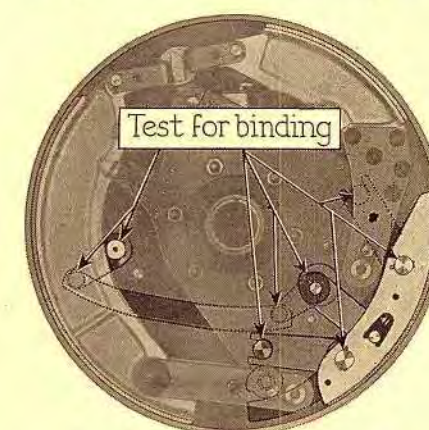
Insufficient release or binding of guide pins or connections may cause hand brake shoes to rattle
