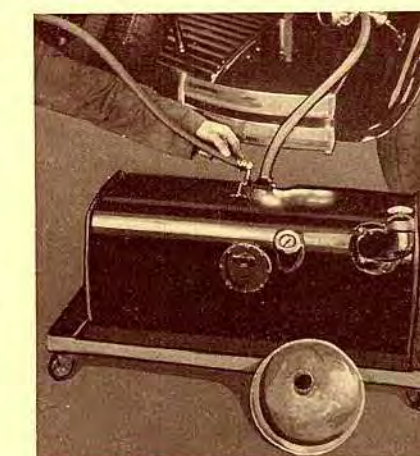
This portable tank and funnel (foreground) simplifies the job of testing gasoline gauges and draining gasoline tanks for repair work on gauges.
