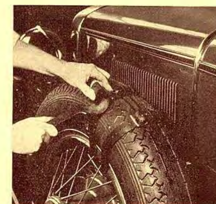
Spare tires will fit snugly in fenderwells if the straps are tightened with this simple tool
