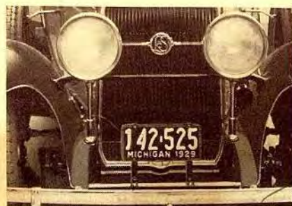
A license plate properly mounted on the new front brackets with which LaSalle cars are now equipped. The brackets are adjustable both in width and in height so as to accommodate plates of various sizes.
