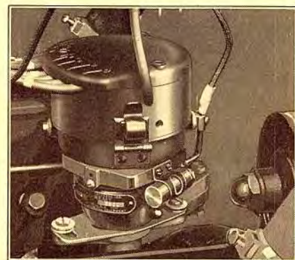
In its new location, the ignition condenser is less affected by the heat than formerly
