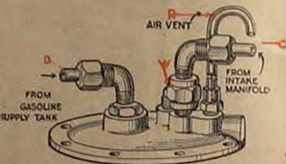
Figure 4 Showing the arrangement of connections on the top of the tank.
