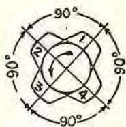
Fig. 10. Illustrates the movement of the cam. Note that the cam moves 90 degrees, or one-fourth revolution each time the crank moves 180 degrees, or one-half revolution.
