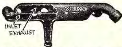
Fig. 20. Wilmo exhaust-heated intake manifold, designed for Fords and other cars. An example of method for heating the mixture just before it passes into the cylinders. The carburetor connects with the lower, or inlet part of the manifold; the exhaust is the upper part, with a plate between. By completely vaporizing the gasoline, no residue is left to seep into the crank case to thin the lubricating oil.
