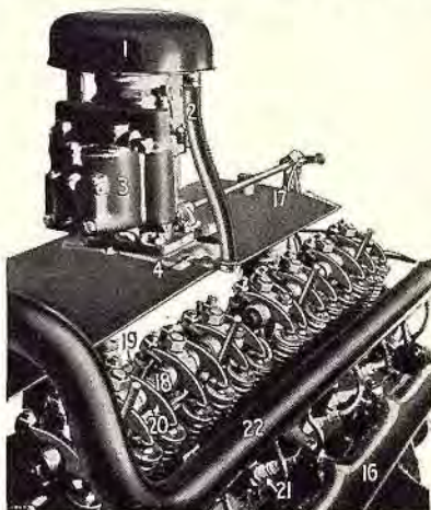
Cover removed showing the accessible overhead valve mechanism of the Marmon sixteen-cylinder engine.
