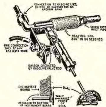
Fig. 17. Heating the priming mixture electrically. A pipe connects with gasoline supply. The primer is screwed into the inlet manifold. Suction of the piston draws in raw gasoline. An electric heating coil connected with the battery heats the gasoline used for priming as it passes into the manifold. There are various electrical methods for heating.
