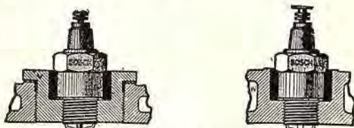
Fig. 3. Correct position of plug in valve cap, but too long a path to cooling water.
