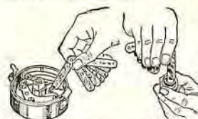
Fig. 22. Method of testing the gap of a spark plug with a thickness gauge (right). Method of testing ignition breaker-contact gap with a thickness gauge when breaker-cam is causing the points to separate (left). The breaker-contact points should be checked for cleanliness and squareness and then set gap as recommended by manufacturer. 3
