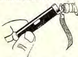
Fig. 32. The Airco tester as applied to the end of a spark plug. Flashes occur in the white gap if there is current. If placed on an insulated wire conducting a high tension, current flashes will occur.
