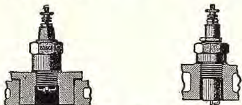
Fig. 1. Valve cap too thick; out of the path of the gas and too long a path to cooling water.
