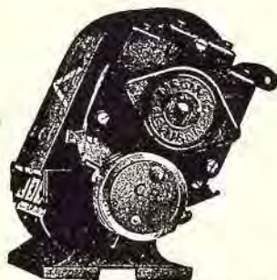
Fig. 3. The Eisemann high-tension magneto, pivoting or rocking advance magneto. The advance and retard are obtained by rocking the magneto bodily on its cradle. Otherwise the magneto is the same as other magnetos. The armature revolves. (Not now manufactured. It is shown in order to exemplify the meaning of a "pivoting or rocking" method of advance and retard.)
