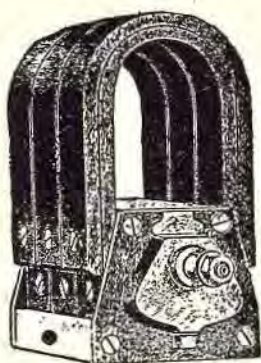
Fig. 1C. The low-tension magneto complete. View shows the drive end of the armature, which is driven at a fixed speed from the crank shaft of the engine, by gear or chains. The direction of rotation of all generators is considered at the drive end.
