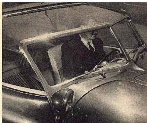
Transparent sun roof over front seat has been retained throughout all versions for experiments in filtering sunlight with different-colored plastics. Rear part of the car's top is solid steel.
