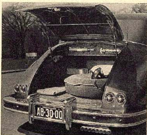
Trunk lid raises hydraulically; so does radio aerial to its right. Inside are fire extinguisher and compressed-air cylinder for filling flat tires. The eight-stack exhaust pipe is just for looks.
